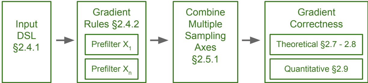
Figure 2.1: Our framework takes as input an arbitrary program expressed by our DSL (§2.4.1), and approximates the gradient by pre-filtering a 1D box kernel along sampling axes (§2.4.2). Approximations along multiple sampling axes are later combined (§2.5.1). Finally, we formally prove our gradient approximation is first-order correct in §2.7 and 2.8, and we also design a quantitative error metric (§2.9) to evaluate any gradient program empirically.
